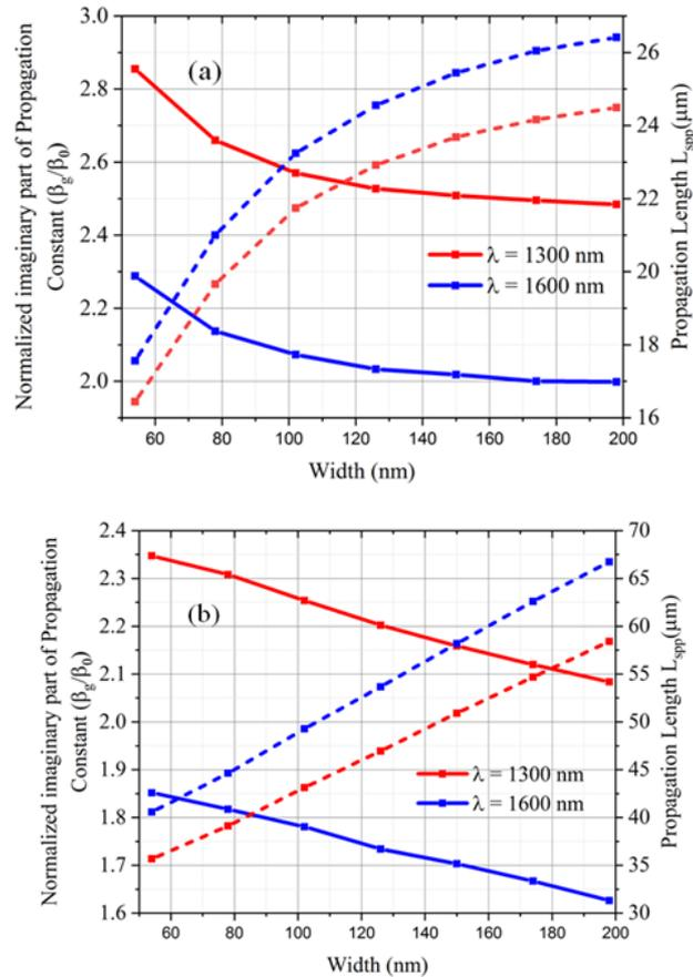
Fig.3 Variation in Normalised imaginary part of Propagation Constant and Propagation Length with Width ( $W_2$ ) of MIM Waveguide for Wavelength  $\lambda=1300$ -nm and 1600-nm for (a) even mode (b) odd mode.
