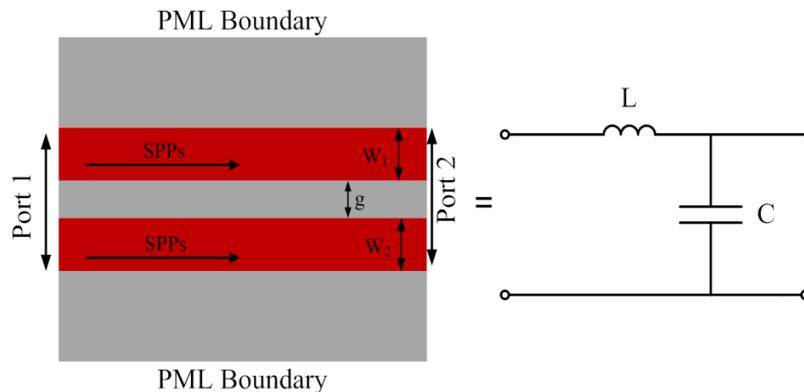
Fig.1 Schematic of Edge Coupled Plasmonic MIM Waveguide
