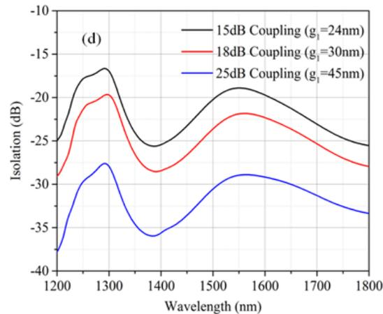
Fig.6 Simulated (a) Return Loss (b) Through port Insertion Loss (c) Coupled port Insertion Loss (d) Isolation (dB) of the Coupler
