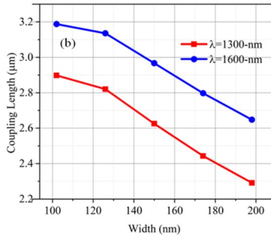
Fig.4 Coupling Length(µm) versus (a)Width ( $W_2$ ) (b)Width ( $W_1$ ) of MIM Waveguide for Wavelength  $\lambda=1300\text{-nm}$  and  $1600\text{-nm}$
