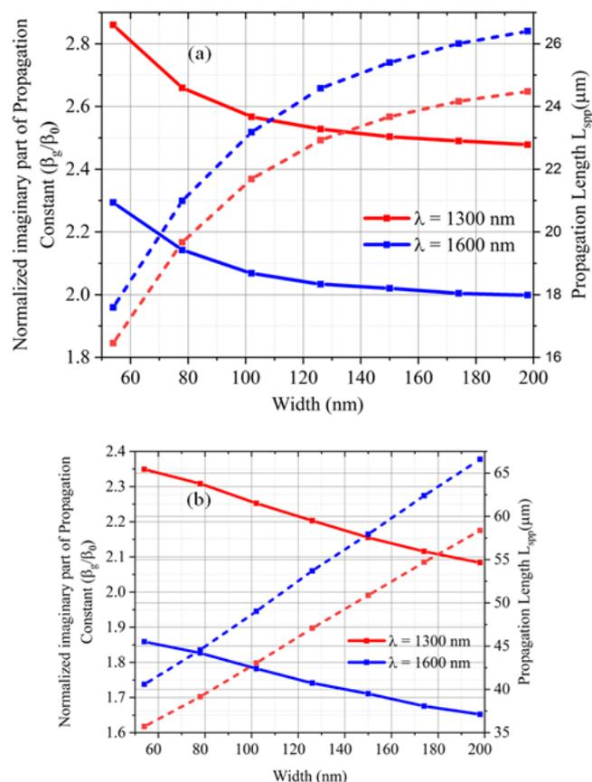
Fig.2 Variation in Normalized imaginary part of Propagation Constant and Propagation Length with Width ( $W_1$ ) of MIM Waveguide for Wavelength  $\lambda=1300\text{-nm}$  and  $1600\text{-nm}$  for (a) even mode (b) odd mode.
