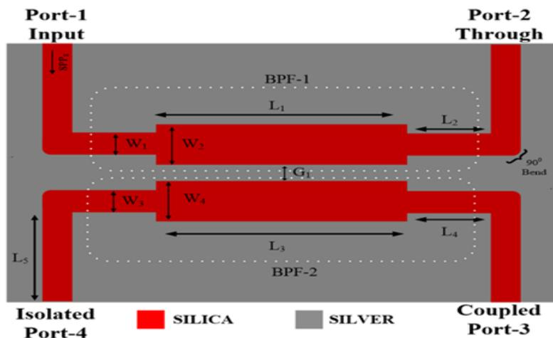
Fig.5 Geometry of the dual band MIMSIR based plasmonic Directional Coupler for fixed widths  $W_1=100\text{nm}$ ,  $W_2=360\text{nm}$ ,  $W_3=100\text{nm}$ ,  $W_4=360\text{nm}$ , lengths  $L_1=2000\text{nm}$ ,  $L_2=500\text{nm}$ ,  $L_3=1900\text{nm}$ ,  $L_4=475\text{nm}$ ,  $L_5=630\text{nm}$ ,  $G_1=60\text{nm}$ .
